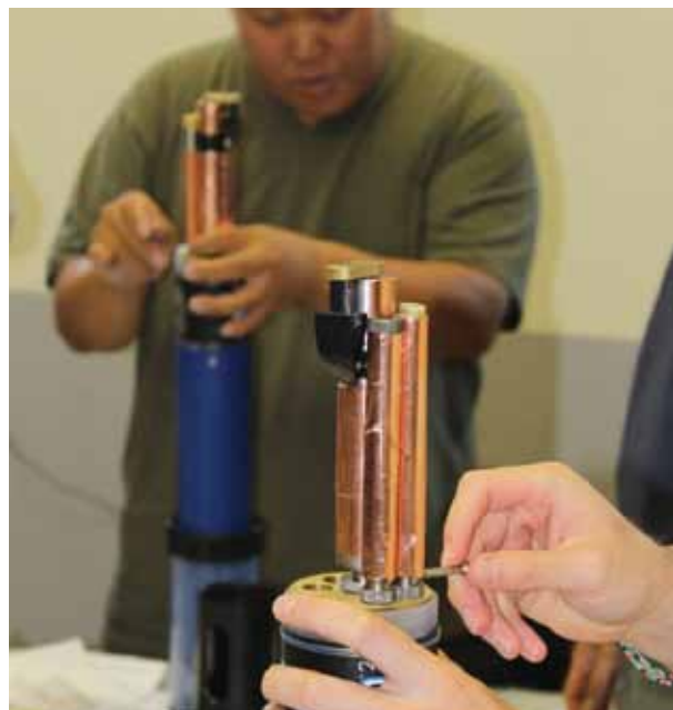
NYC DEP staff learns how to set up and calibrate the EXO2 sonde and sensors.
