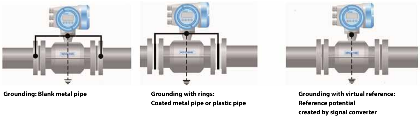
Figure 2 – A diagram comparing standard grounding methods with virtual reference
