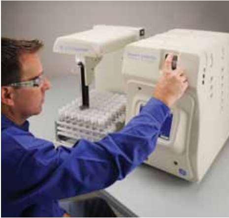
The Sievers InnovOx has a Web interface for remote monitoring
