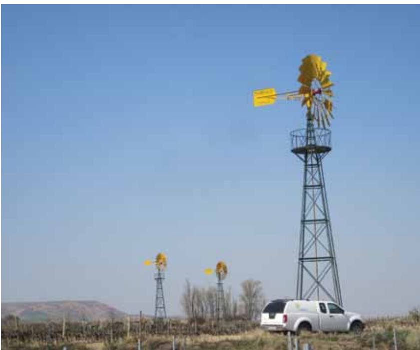
The windmill automatically stops in case of too strong wind
